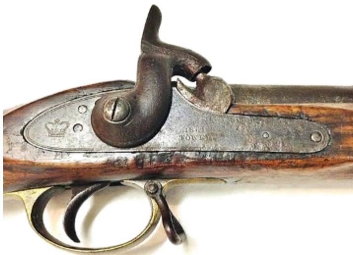
*Detail: Lock plate marked with a British Crown and "1861/TOWER". "Tower" was a quality inspection mark used by the British government facility at the Tower of London*
